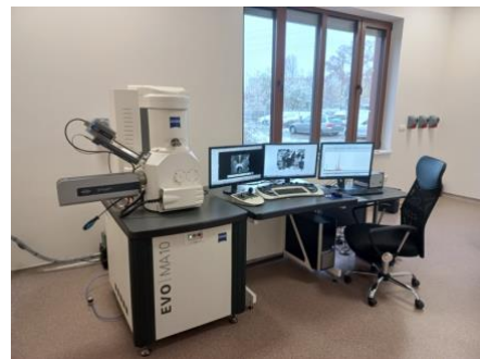
Figure 1: The cryogenic set-up, the cryostat and the scanning electron microscope (SEM, EBSD)
